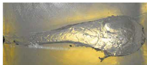
Simulated wound cavity in ballistic soap - .300 Win. Mag. SPEED TIP PRO at 350 m
